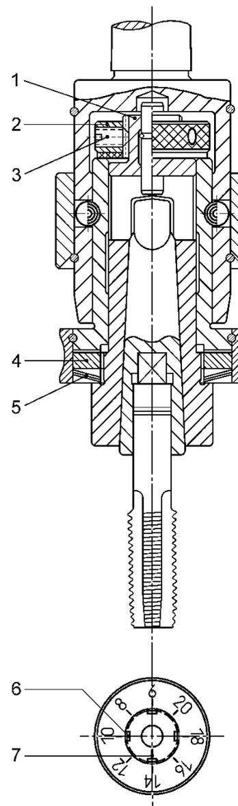
If, for example, you want to cut a thread M12 in steel 70-2 with tapping adaptor GE34-MT3, the setting for this according to the table on page 3 is IV/12. IV refers to the position of the built-in cup springs (5) and 12 is the setting number on the adjusting nut (2).
