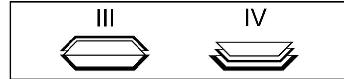
Installation position of disc springs
