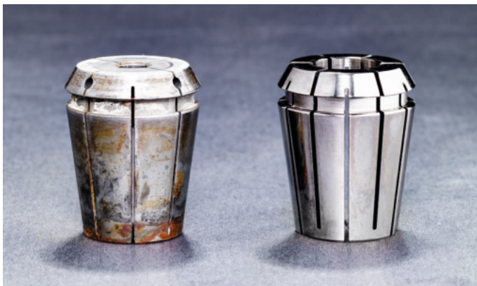
Two collets each after 4 months of use: The left one without coating – the right one with FAHRION|Protect
